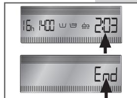
**DELAYED START:** This function allows the start of the wash cycle to be delayed by up to 16 hours. Press button **B** repeatedly until the required delay time appears on the display. Icon h will flash on the display until the wash cycle starts.
