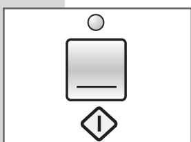
**START:** During the phase for selecting programs and washing options, the start LED stays off. To confirm the selections and start the wash cycle, press "Start" button **H**. The LED will light up.
